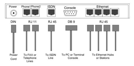
Figure 0-1, Hypertec ISDN 10T Router Rear Panel
